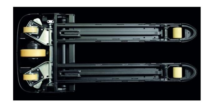
5-wheel configuration = support the drivers application = less accidents and productivity = reduced handling costs / pallet
